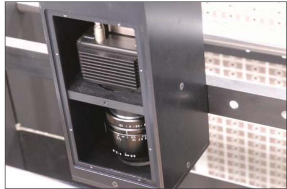
Piranha2 camera in action capturing high resolution images for the visible inks integrity analysis.
