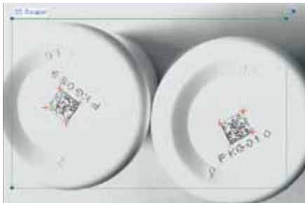
DOT PEEN 2D CODES ON PLASTIC
