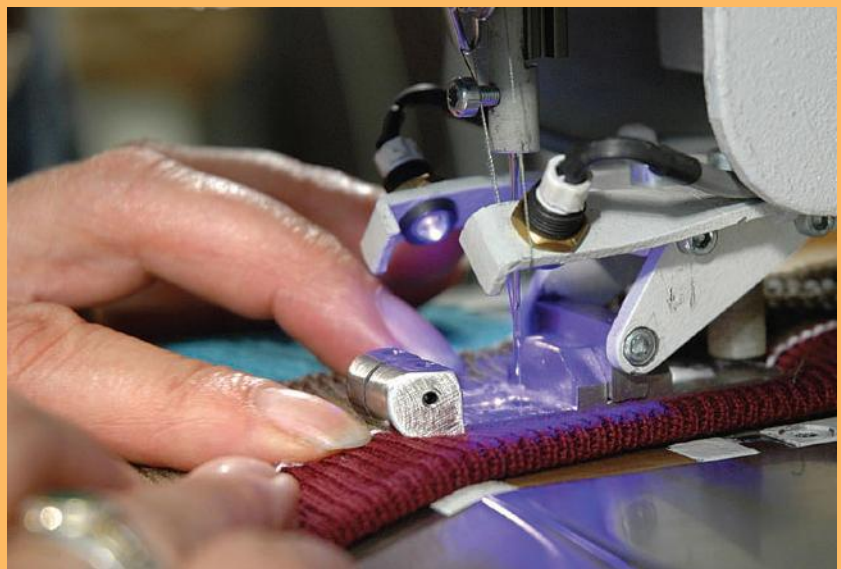
By using a vision-guided system based on a sewing machine, an operator can link together two different fabrics without the need to use a traditional linking machine.
